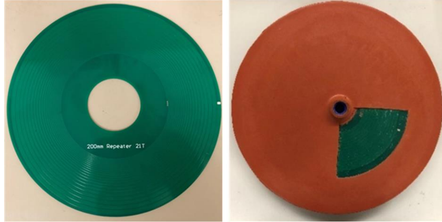
PCB resonators. (Left) double-layer winding. (Right) embedded in an insulator shed.
